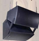
The horizontal fly kit (model **IB-HFK**) facilitates the horizontal array hanging of 2 same-size enclosures with up to a 45° splay between cabinet edges. Each kit includes 2 planar spacer plates, 2 flykit spacer brackets and 4 M10 eyebolts. To horizontally array 3 same-size enclosures, simply utilize 2 horizontal fly kits; to horizontally array 4 same-size enclosures, use 3 kits; and so forth.
