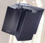
Community's universal planar kit (model **IB-UPK**) allows you to create clusters of 3 enclosures from the iHP3500, iHP1500 or iHP1200 series. When clusters of 3 same-size enclosures are created, up to a 45° splay between cabinet edges is possible. When
