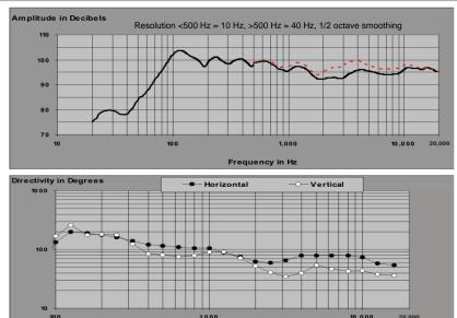
Frequency in Hz Recommended Power: 400 to 625 WRMS<sup>1</sup> at 8Ω Recommended High-Pass Filter: 55 Hz, 24 dB/octave
